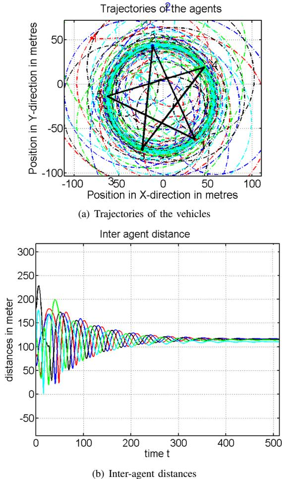
Fig. 6.  $\{5/2\}$  formation configuration with unicycle model
