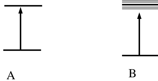
Fig. 8.3 Fig. A shows transition from ground to excited state. Fig. B shows excited state level broadened.
