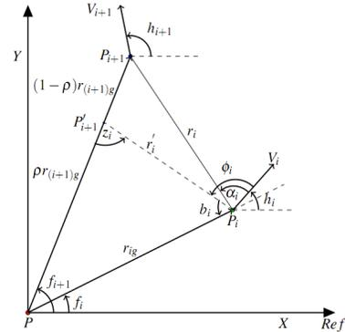
Fig. 2. Vehicle Formation geometry [9]
