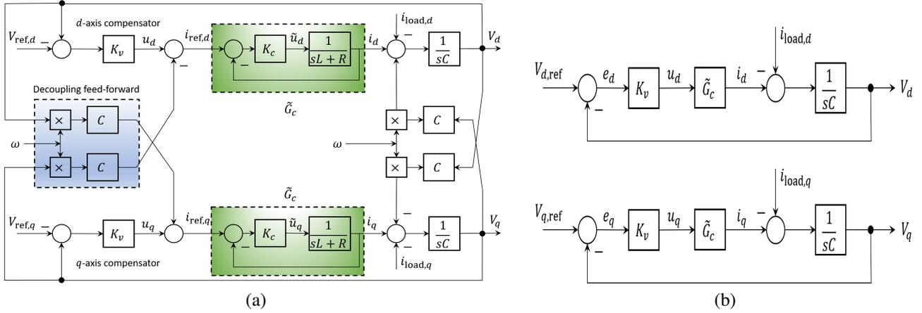
Fig. 3: (a) Control model of a single full-bridge DC-AC inverter. The feed-forward term decouples the dynamics of  $i_d$  and  $i_q$ . (b) Control model with decoupled loops.
