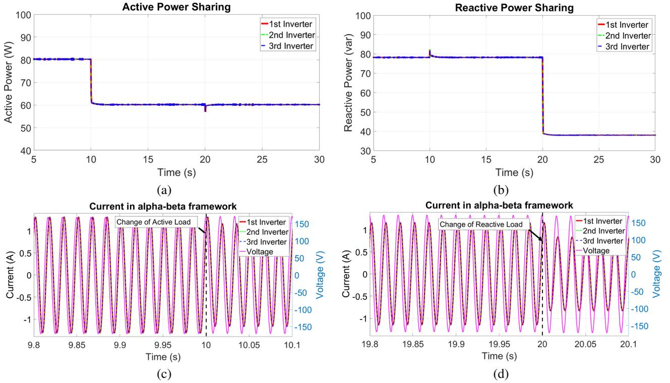
Fig. 6: (a) Equal sharing is maintained during sudden change in (a) active and (b) reactive loads. Output voltage and current waveforms during changes in (c) active and (d) reactive loads. The proposed control scheme exhibits precise active and reactive power sharing capability, while ensuring voltage regulation in presence of uncertain and time-varying load.
