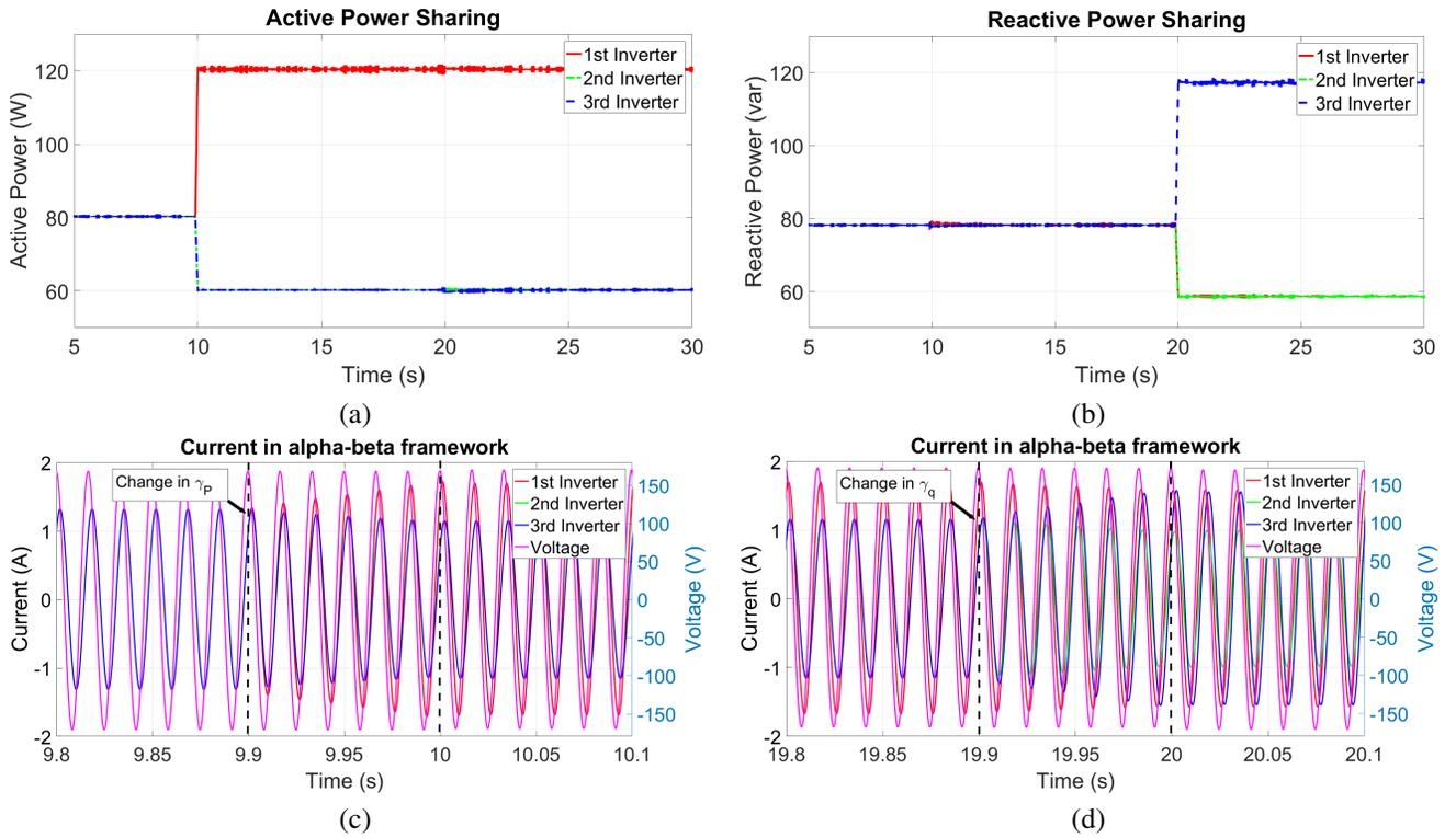
Fig. 5: (a) Active and (b) Reactive power outputs of the inverters. Output voltage and current waveforms during change in (c) active and (d) reactive power sharing requirement. The proposed control scheme exhibits precise *dynamic* active and reactive power sharing capability, while ensuring voltage regulation in presence of uncertain load.
