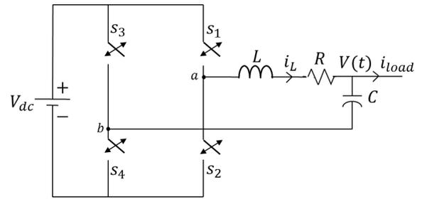
Fig. 2: Circuit representing a full-bridge inverter. The AC-side current is given by  $i_{load}$ . The switches  $s_1, s_2, s_3$  and  $s_4$  control the AC-side voltage  $V(t)$ .
