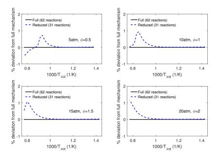
Figure 2: Ignition delay time deviation from the full mechanism for  $H_2/air$  mixture.
