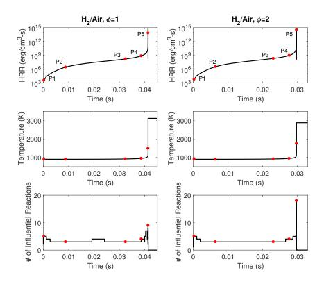
Figure 1: Calculated heat release rates (HRR), temperature profiles, and the number of influential reactions for  $H_2/air$  mixture with the initial condition of 20 atm and 900 K. Highlighted are five points (P1-P5) during the time evolution.
