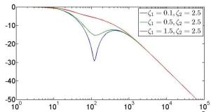
Fig. 5: Bode magnitude plots of the closed-loop plant  $\tilde{G}_c$  for various  $\zeta_1$  values.  $\tilde{\omega}$  is chosen to be  $600\pi$  rad/s. Note that a relatively larger value of  $\tilde{\omega}$  is in accordance with choosing a fast inner-current controller.
