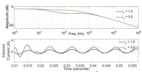
Fig. 9: Bode plots of inner-shaped plants  $\tilde{G}_c$  and inductor currents for different  $\zeta_1$ . While the average (or DC) current remains the same as desired, the smaller values of  $\zeta_1$  result in relatively smaller magnitudes of 120 Hz ripple in inductor currents.
