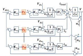
Fig. 6: Control framework for a many-converters system. Note that in the proposed implementation, we adopt the same outer controller for different converters, i.e.,  $K_{v_1} = K_{v_2} = \dots = K_{v_m} = K_v$ .
