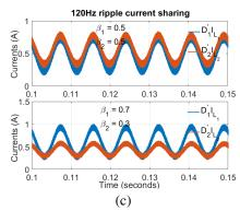
Fig. 8: (a)Voltage regulation in presence of modeling uncertainties and 120 Hz ripple at the output. The inner-outer controller regulates the output voltage to the desired voltage,  $V_{des} = 24$ V. (b) Average current (power) sharing between two converters in the ratios 1:1 and 7:3. (c)  $\omega_0$  average ripple sharing between two converters in the ratios 1:1 and 7:3.
