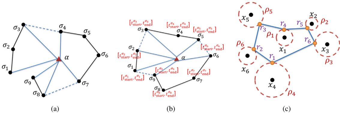
**Fig. 1.** Schematic of (a) Single-depot VRP with  $n = 9$  customer locations, represented as black dots. (b) Single-depot VRPTW. (c) Single vehicle returning CETSP, where each location  $x_i$  has a radius  $\rho_i$ , within which a vehicle can ‘visit’ the customer. The orange dots indicate the visit points  $r_j$  within the allowable radius  $\rho_i$  for each customer  $i$ .
