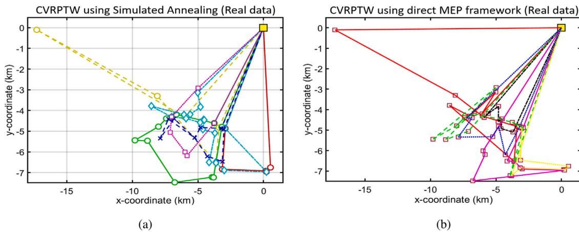
Fig. 11. Performance of the simulated annealing (SA) and the proposed MEP approach for 60 customers Gurugram data with three service time-windows (a) SA: Run-time 49.5 s, (b) MEP approach: Run-time 44.1 s.
