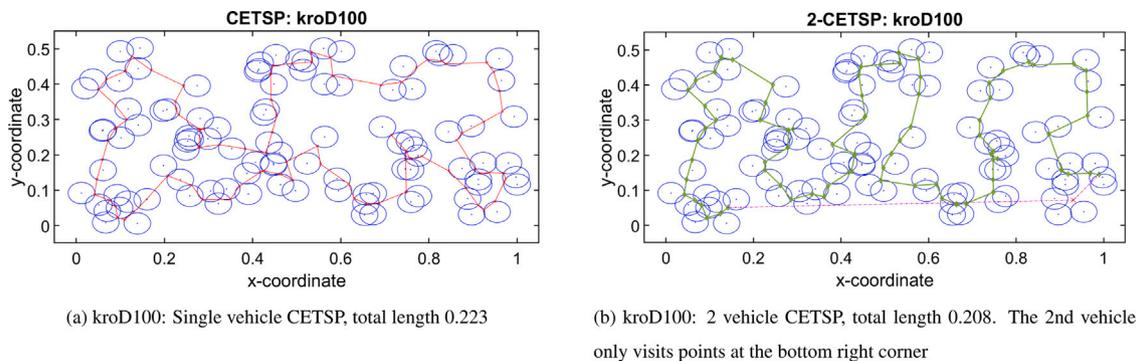
Fig. 8. Illustration of the MEP approach solutions for CETSP instances, with a single vehicle and multiple vehicles.
