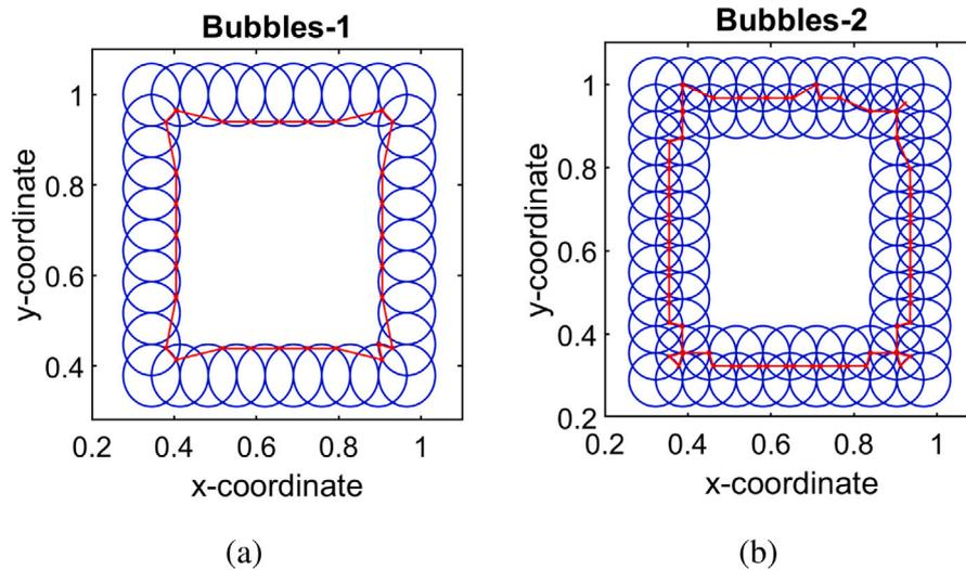
Fig. 7. CETSP solutions on the Bubbles benchmark instances. (a) Bubbles-1: Finds optimal solution, except for the tiny 'hook' at the right-bottom corner. (b) Bubbles-2: MEP uses the intersection of two circles to reduce travel distance.
