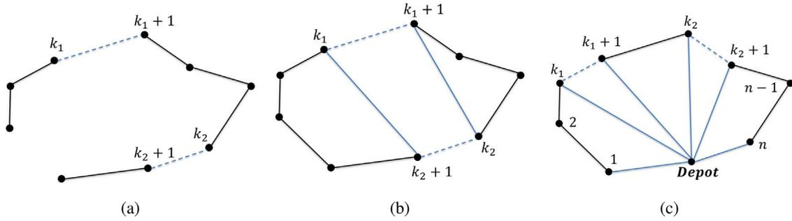
Fig. 5. Schematic of a (a) Non-returning  $m$ TSP with  $m = 3$  and  $R = \{k_1, k_2\}$ , equivalent to creating three clusters and Hamiltonian paths in each cluster; (b) Returning  $m$ TSP with  $m = 2$  and  $R = \{k_1, k_2\}$ , equivalent to creating two clusters and creating tours within each cluster; and (c) Single-depot VRP with  $m = 3$  and  $R = \{k_1, k_2\}$ . The dashed blue lines indicate the removal of links, while solid blue lines indicate the addition of links.
