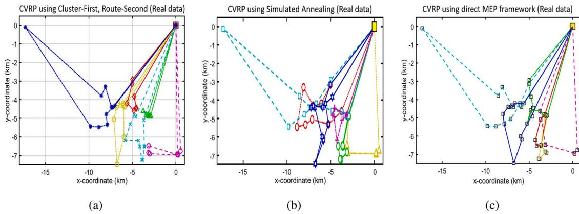
Fig. 10. Comparison of the proposed simultaneous clustering and routing approach with the cluster-first route-second method and simulated annealing (SA) for the 60 customers Gurugram data. (a) Cluster-first route-second-Run-time: 46.6 s, Sq. total length: 789.78 km. (b) SA-Run-time: 51.2 s, Sq. total length: 706.46 km. (c) MEP approach-Run-time: 17.08 s, Sq. total length: 552.44 km.
