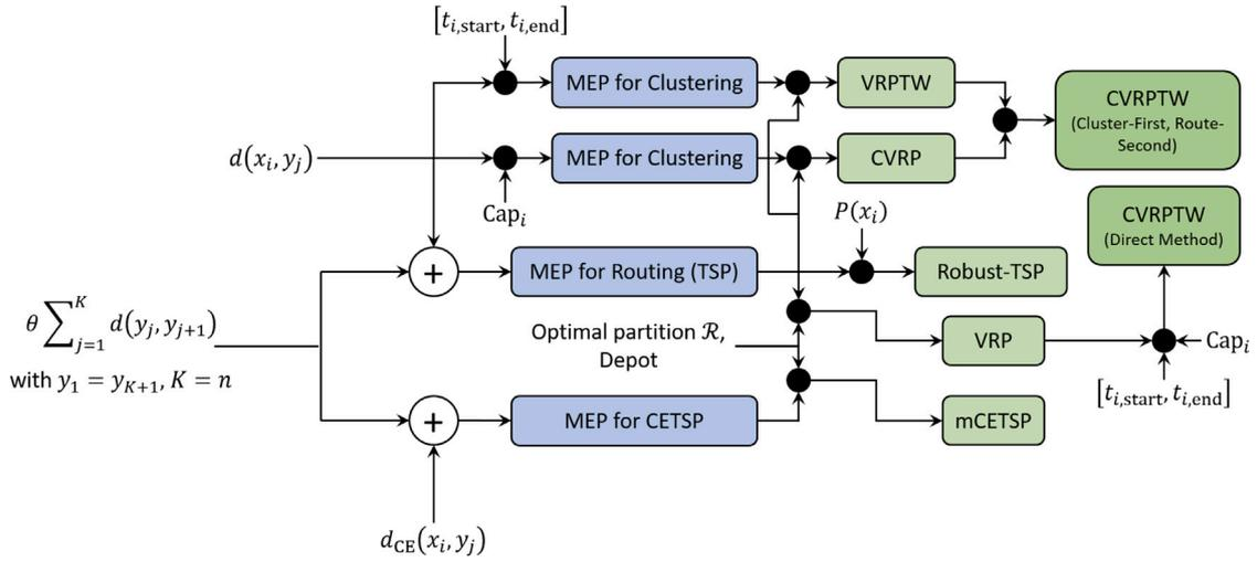
Fig. 2. Overview of MEP methodology for solving VRP and its variants — the blue colored textboxes represent the solution approach, while green colored textboxes depict the problems being solved.
