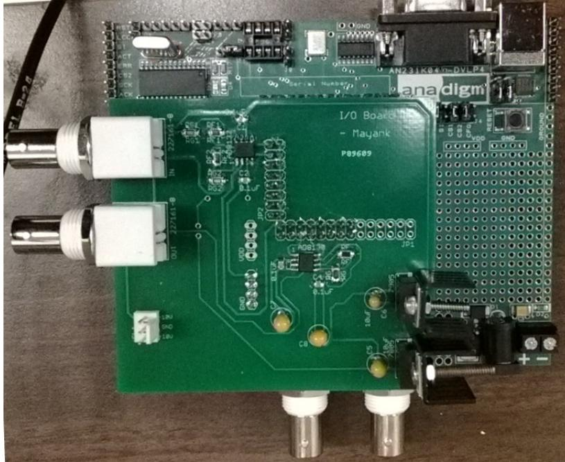
Figure 2.2: A custom designed PCB for interfacing FPAA with the AFM
