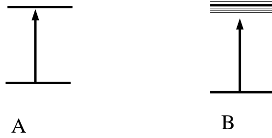
Fig. 3.13 Fig. A shows transition from ground to excited state. Fig. B shows excited state level broadened.
