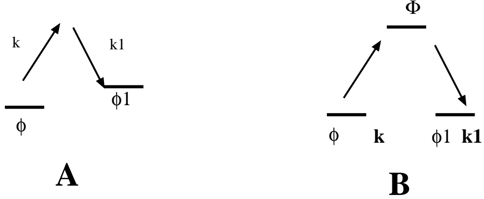
Fig. 3.8 Fig. A, depicts stimulated Raman scattering, incoming photon at wavevector k scatters to wavevector k_1 by stimulation. Fig B, depicts a three level Rayleigh process, where initial atomic level \phi absorbs photon k and moves to \Phi where CM coordinate gets photon momentum. k_1 is emitted and we return to \phi_0
